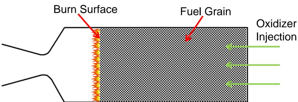
The project objective is to conduct regression rate experiments of an axial-injection, end-burning hybrid rocket motor and use a modified ablative model to describe the experimental results.
