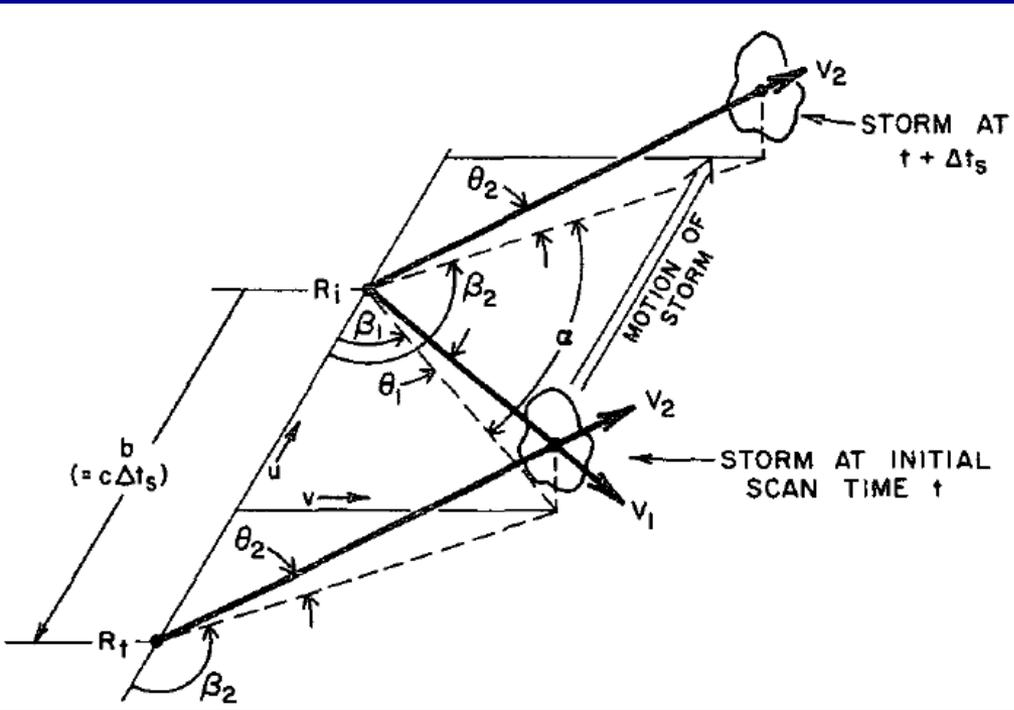
**Geometry of the (synthetic) dual-Doppler technique**
