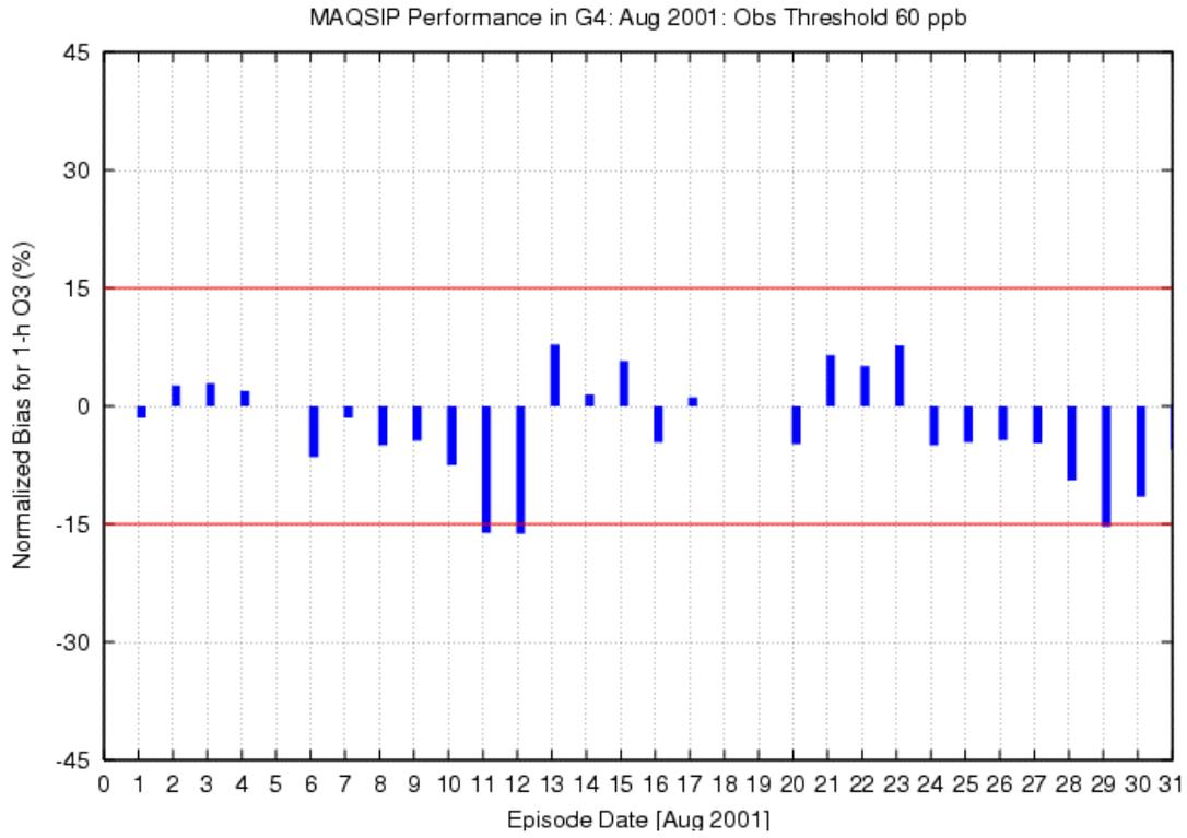
**Figure 8a.** MAQSIP-RT 24-hour forecast (15km SE grid) normalized bias using 60PPB cutoff.
