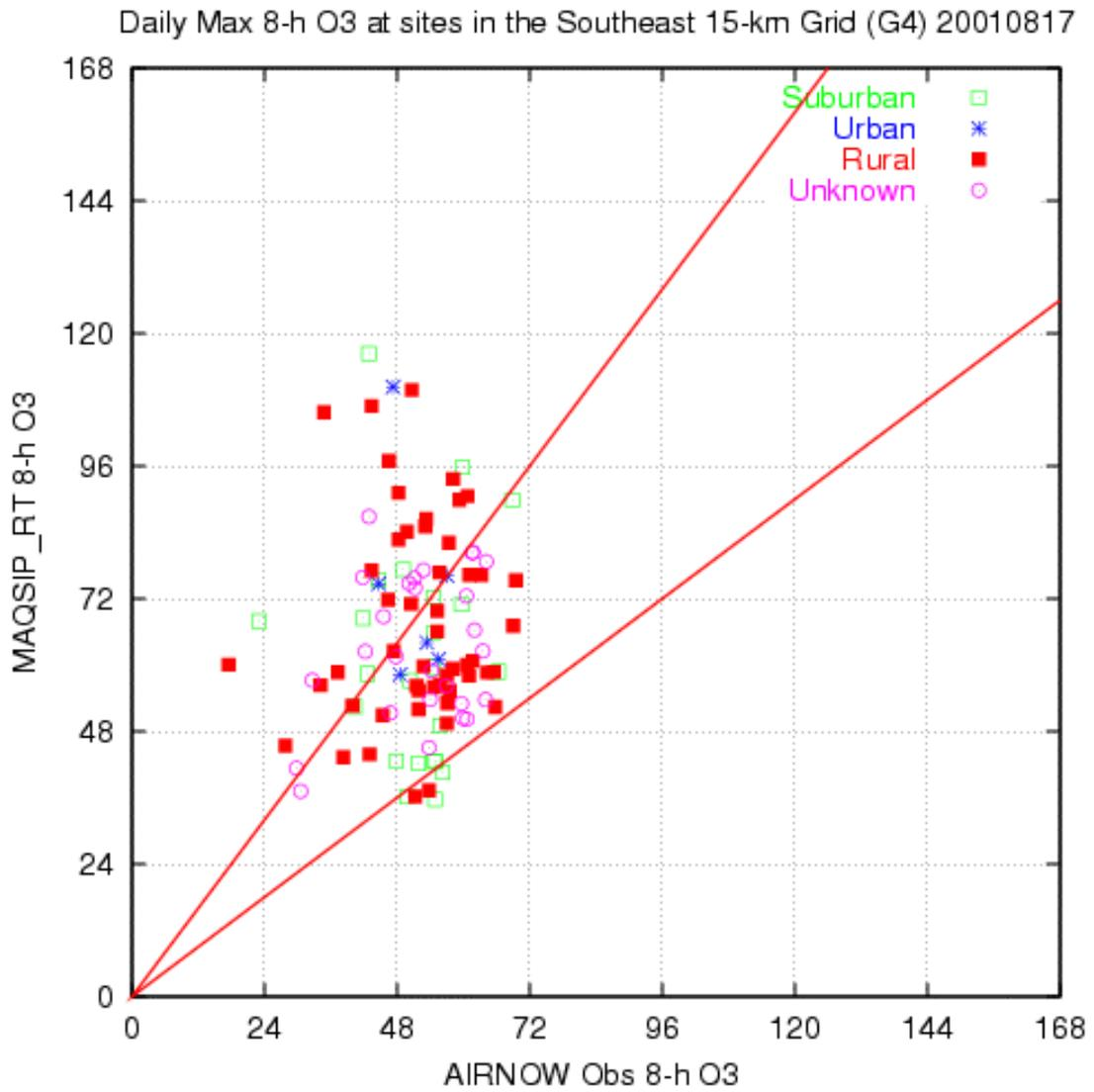
**Figure 6b.** Scatter plot of 24-hour forecast versus observed ozone for Aug 17<sup>th</sup>, 2001, MAQSIP-RT 15km SE grid.
