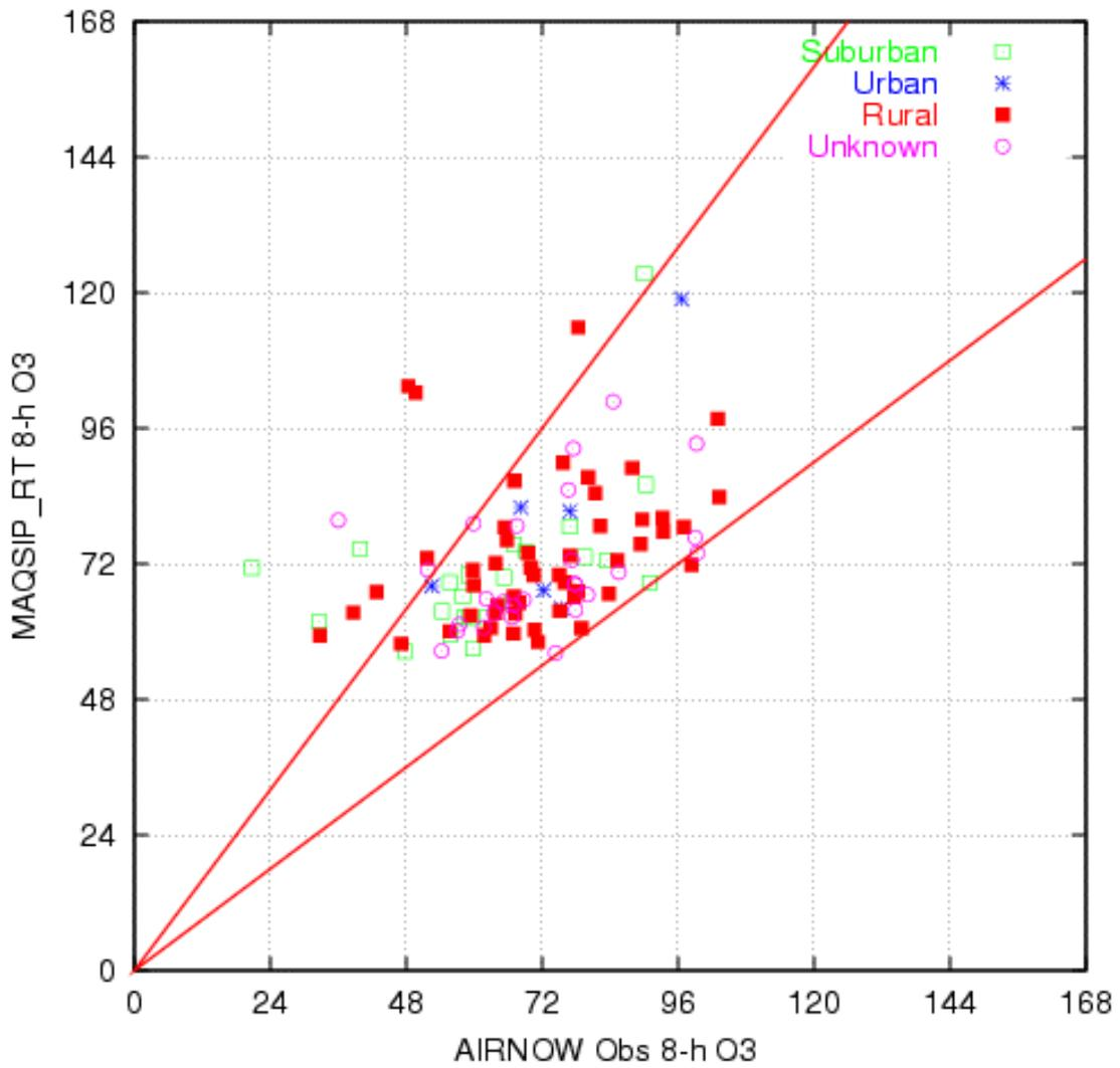
**Figure 7b.** Scatter plot of 24-hour forecast versus observed ozone for Aug 23<sup>rd</sup>, 2001, 15km MAQSIP-RT.
