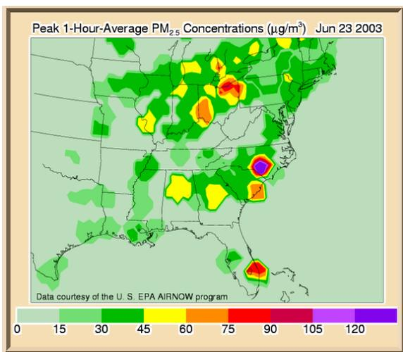
**Figure 2.** An example of our new capability to generate regional contour maps of PM<sub>2.5</sub> in near real time, using EPA-AIRNOW continuous data of 462 sites.
