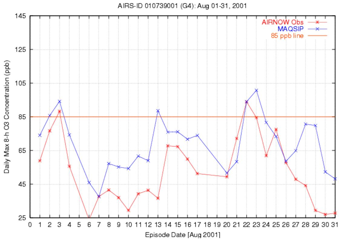
**Figure 4c.** August 2001 time-series of daily *maximum* 1-hour-ave (top) and 8-hour-ave (bottom) MAQSIP-RT 15km SE grid forecast versus observed ozone for the Tarrant City (Jefferson County) monitor.
