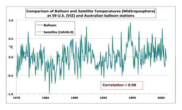
Fig. 2: Average temperature variations measured at 59 radiosonde stations in the U.S. (VIZ manufacturer) and Australia.
