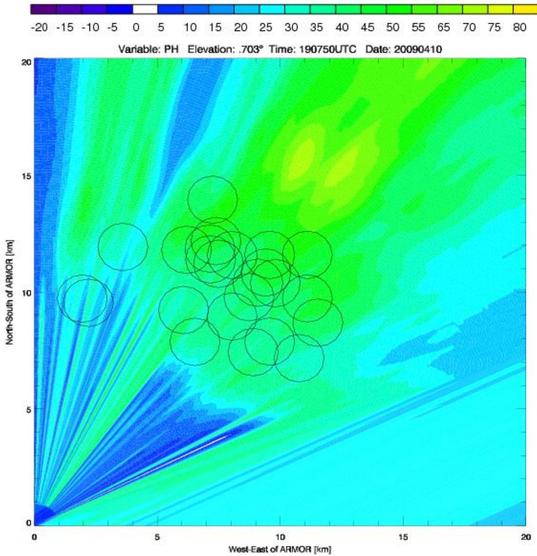
Figure 4.6: Same as Figure 4.2 except contoured  $\Phi_{dp}$  ( $^{\circ}$ ).
