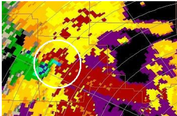
Figure 10. 2102 UTC 0.5 deg storm-relative velocity (BMX) showing gate-to-gate maximized (magnitude > 50 \text{ kt} , > 25 \text{ m s}^{-1} ) inbound and outbound velocities.
