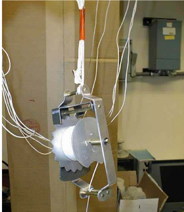
FIGURE 8. PAYOUT REEL ATTACHED TO PARACHUTE.
