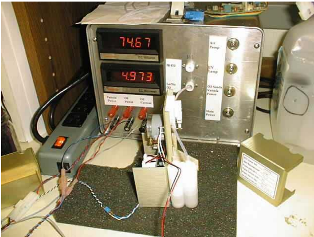
FIGURE 3. OZONESONDE TEST UNIT : 2Z SONDE RUNNING ON 5 MICROAMPS OZONE
