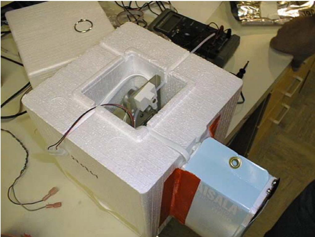
FIGURE 7. TOP VIEW OF OZONESONDE PLACED INSIDE BOX.
