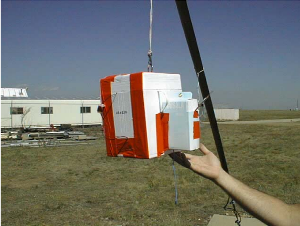
FIGURE 10. OZONESONDE TAPED UP & SAMPLING SURFACE AIR FOR 5-10 MINUTES.
